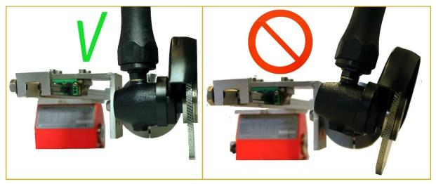
Make sure the cutting disc is attached with a 90deg angle to the surface.
