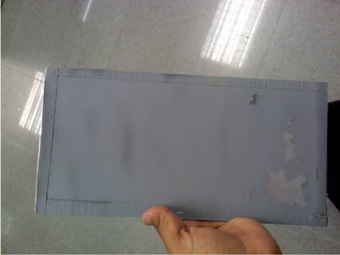
Interzinc 12 after Mud Cracks
