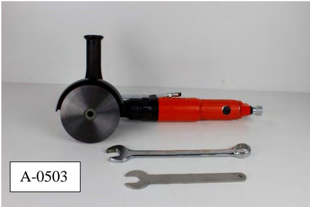
When attaching and removing the Weld Seam Disk (A-0503) to the A-0105 Air Tool you will need the following accessories:
