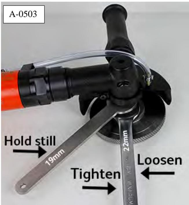
To complete the tightening of the Weld Seam Disk, use both 22mm and 19mm Spanners.
