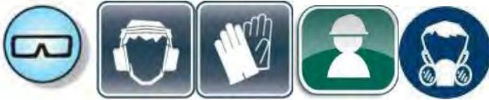
Always wear the necessary protective equipment when using this equipment. Safety goggles or face shield, gloves and hearing protection are required. Ensure all clothing is close fitting to prevent becoming snagged in moving parts.
